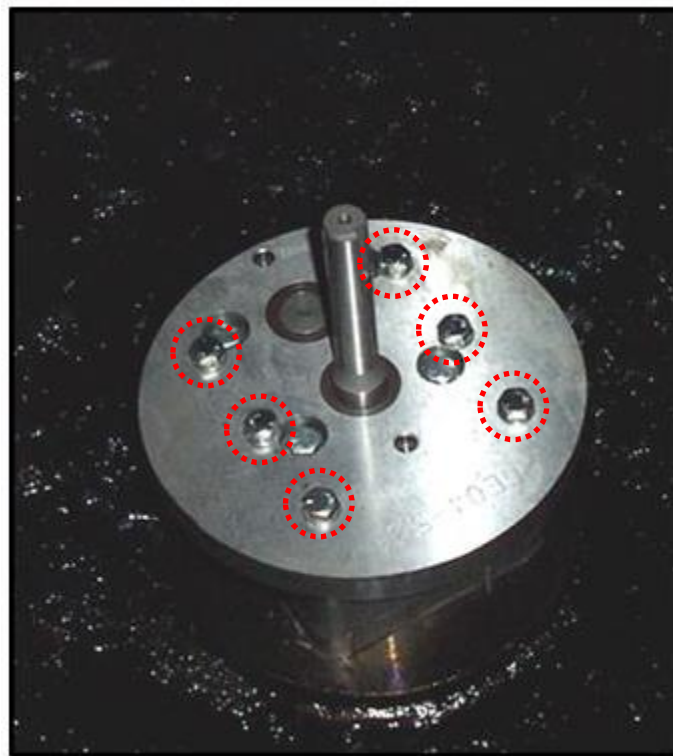
Figure 6-7 Unbolting the Material Pump
